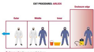
Enclosure edge: Vacuum coverall, footwear Airlock inner stage: Wipe mask, brush boots, clean equipment Middle: Remove outer coverall (retain for re-entry or discard) Outer: No action Outside airlock: Remove RPE
