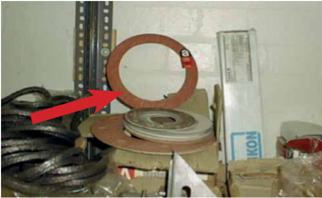
CAF – Compressed Asbestos Fibre.
